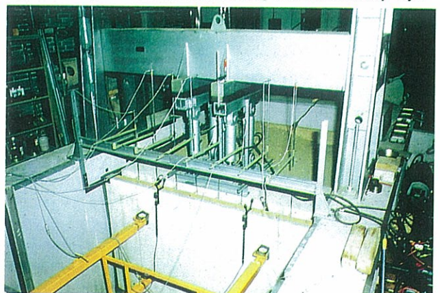
Figure 15 Large-scale tests for developing the bituminous slip-layer
