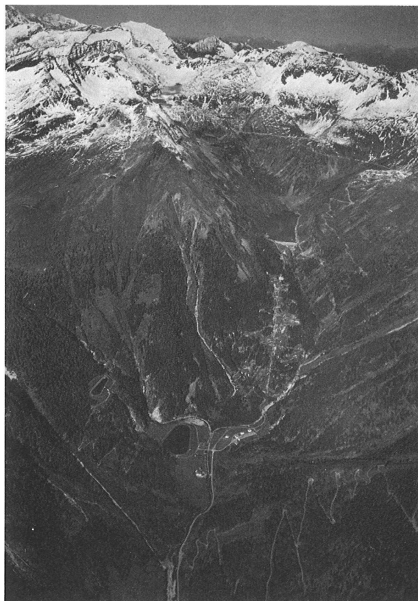
Fig. 34. Innerfragant valley head. From the top downwards: Hochwurten reservoir (K2), Wurtenalm reservoir with penstock of Wurten stage (K3) as well as powerhouse (K3+K4) and Innerfragant compensation reservoir (K6) and Haselstein stage (K5); construction road to the Oscheniksee reservoir (K4) in the bottom right-hand corner (released for publication by the BMFLV under ZL. 13080/254 — 1. 6./79)
